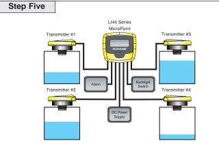
**A. Factory Calibration:** Out of the box, the indicator is factory calibrated to interface with (4) SOURCING two-wire loop powered level transmitter inputs and display percentage of measured span on each channel. The following describes the indicator functions as delivered under factory calibration:
