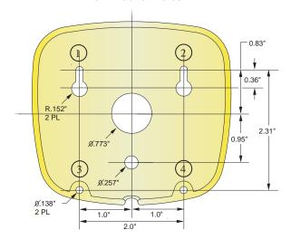
Use the above hole dimensions for purposes of drilling the (4) wall bracket mounting holes.
