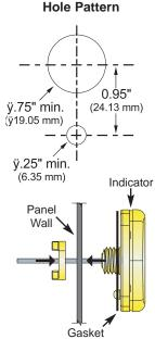
**C. Wall Mount:** Follow the below steps to install the indicator in a wall mount configuration:
