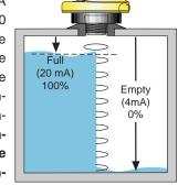
C. MicroCal Calibration: To customize engineering units, configure FET alarm set points from level transmitter, level switch or leak detection switch inputs, and/or linearize the volumetric measurement of odd shaped tanks, use the MicroCal calibration kit. MicroCal calibration users should now go to the MicroCal Calibration Kit LI96 Series Owners Manual for programming instructions. Once calibrated, return to this manual and continue starting with the Installation Section.
