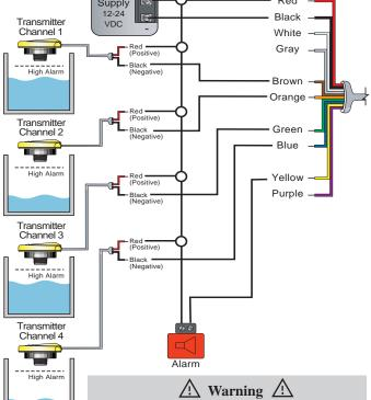
B. Wiring the LI44-1001 to (3) Level Transmitters, (1) Leak Switch and (1) Alarm (Note: Switch and Alarm Functions Require MicroCal)
